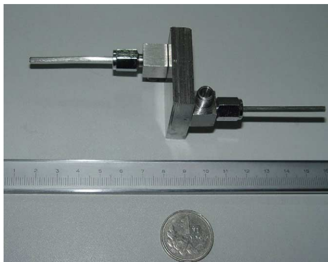
Fig. 4. Photograph of the assembled reformer.
